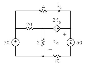
Fig. 3. Example circuit 3.
